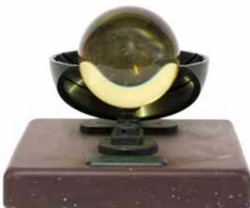
Lot 136 SUNSHINE RECORDER, c.1920s, a sunshine recorder by C Dales & Sons Bournemouth, the thick slate base set with brass fittings comprising a calibrated adjustable graph paper holder and 4in glass sphere, loosely mounted on an adjustable rest, maker's/retailer's plate to front, registration number 366565, 23cm square £200 - 300
